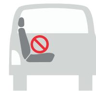
If the front passenger seat is in use, please push it back as far as possible and follow the instructions in your vehicle manual. Disable the front passenger airbag! If this is not possible, the usage of a child car seat on this seat is not permitted. Use the vehicle type list of your manufacturer to check which vehicle seats are suitable for child car seats.
