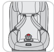
Insert the two buckle tongues (C) of the harness strap (G2) and connect it to the belt buckle (D) until you hear a clear „click“ sound.
