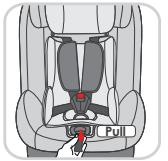
**WARNING:** There should be no more than a finger's width between the body and straps.
