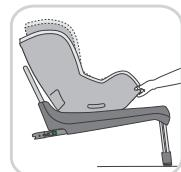
To turn the seat, you must press the rotate button and turn the seat at the same time.
