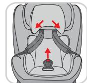
Reach under the cover at the bottom of the seat and pull it slightly forward and upwards. Now pull the cover over the buckle.
