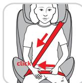
Make sure that the diagonal belt runs exactly and does not run too close to the child's neck. All straps must fit tightly against the child and must not be twisted.
