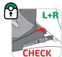
Only a proper fixing of **BOTH TERMINALS** ensures that the seat is secured properly and offers full protection to your child in the car!!!
