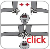
Insert the two buckle tongues (C) of the harness strap (G2) and connect it to the belt buckle (D) until you hear a clear „click“ sound.
