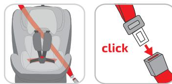
Pass the diagonal strap of the 3-point safety belt through the blue belt guides at the back of the car seat to the buckle.
