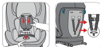
You can then release the harness straps (G2) and the shoulder pad straps (SG) from the adjuster and insert the two strap ends through the shoulder strap guides (G1) pull out.
