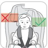
The headrest must be adjusted so that the distance between the shoulders of the child and the headrest does not exceed 3 cm (about 2 finger widths).
