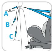
Now take the Top Tether (TT) and guide it under the head rest along to the appropriate Top Tether anchor point of the car. This can be found in the instruction manual of the car.
