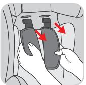
Open the seat belt buckle (D) and the belt system (G).
