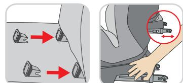
The ISOFIT mounting points are located between the seat and the backrest of the car seat.
