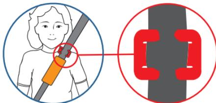
Make sure that the lap belt runs under the fixation lugs (C) on both sides and that the diagonal belt leads only under the fixation lugs (C) on the side of the belt buckle (Q).
