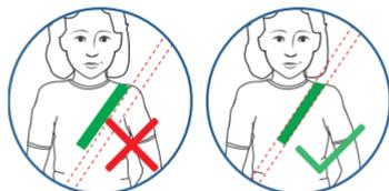
In some vehicles, the diagonal belt does not run optimally over the shoulder area of your child. Always check that the diagonal belt is in the correct position when using it as a booster seat. If the diagonal belt does not run within the intended range, please use the supplied flexible belt guide.
