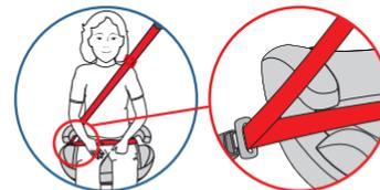
Make sure that the lap belt runs under the fixation lugs (C) on both sides and that the diagonal belt leads only under the fixation lugs (C) on the side of the belt buckle (Q).
