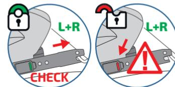
Only a proper fixing of BOTH TERMINALS ensures that the seat is secured properly and offers full protection to your child in the car!!!
